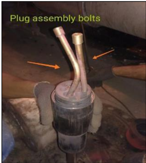
Upgradation of BFP RC valve trim set from single stage to multistage
