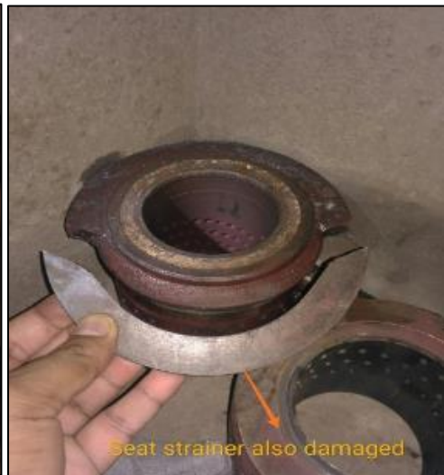
Upgradation of BFP RC valve trim set from single stage to multistage
